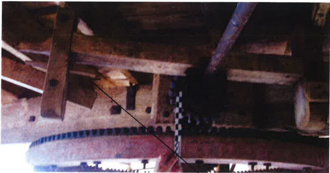
Right hand gear which drives the apple mill.
